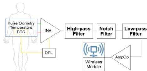
**Fig. 2. Data acquisition system.**
