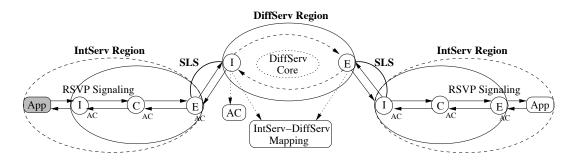
Fig. 1. Intserv/Diffserv integrated solution
