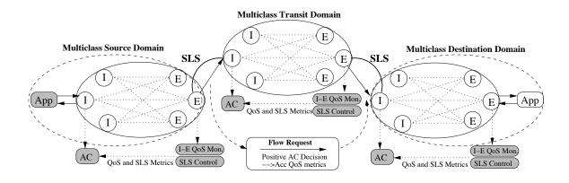
Fig. 4. Distributed monitoring-based AC approach
