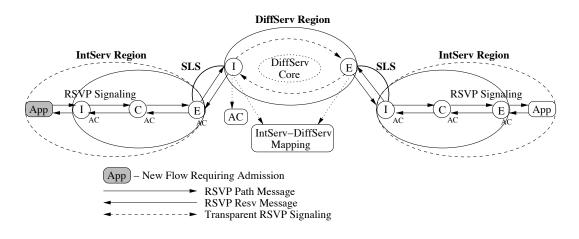
Figure 1. Intserv/Diffserv integrated solution
