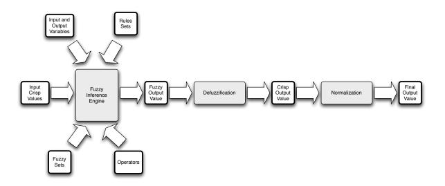
Figure 2: Architecture of the unified QoS metric fuzzy controller.
