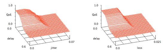
(a) Delay and jitter; (b) Delay and loss
