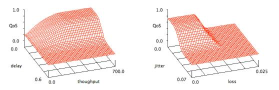
(c) Delay and throughput; (d) Jitter and loss
