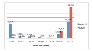
Fig. 7. Packet sizes and bytes (%)
