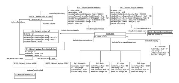
Fig. 4. SLS example diagram for VoIP service
